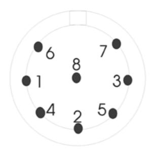
Pin 1 serial data out, bar code input
