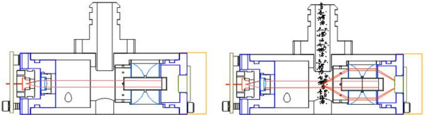
Clean air and particulate scatter conditions in the MD engine
