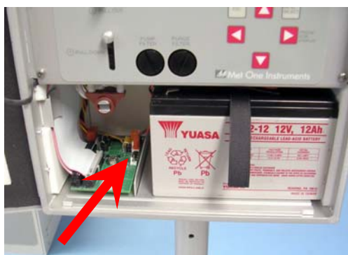
Internal battery and 3620 PCB battery harness connection
